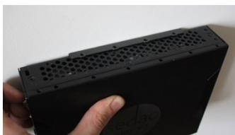
4) Position PRO-V3 player over the top of the mounted plates, with the lips on the plates covering either edge.
